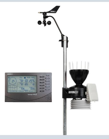
The Cabled Vantage Pro 2<sup>™</sup> is the cabled option for data logging along with a 6510USB data logger, however this is a special-order item and may take 8-10 weeks to arrive.
